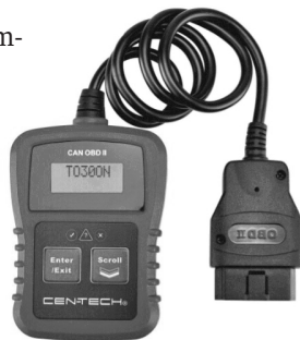
An inexpensive handheld OBD-II reader available at auto parts stores.
