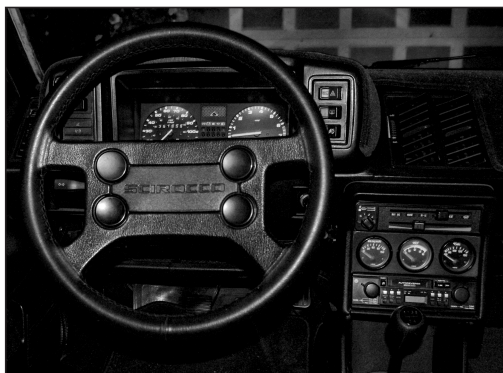
Toggle switches flank the instrument panel with oil temp, oil pressure and volt meter gauges in a console ahead of the shifter.
