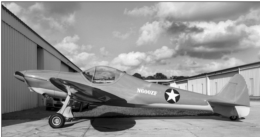
The VanTreurens' Silence Twister, a German ultralight designed for amateur construction from a kit.
