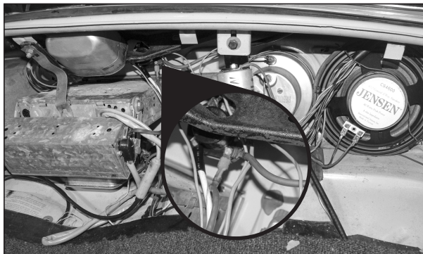
ABOVE: A bad electrical connection, inset, shows the red wires joined at the headlight switch had caused the problem. BELOW: The tiny illuminated generator light signified trouble.
