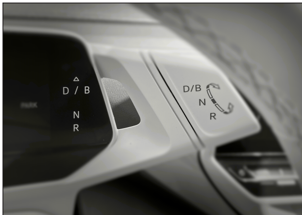
The ID.4's driving mode shifter is situated behind the steering wheel.
