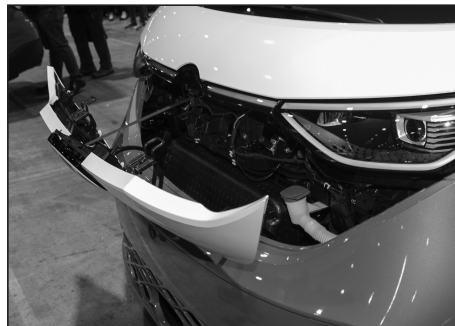
Gear positioned behind the front lid allows for more foot room inside the ID. Buzz.
